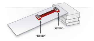
Friction is the resistance met when one surface slides over another; this affects movement (see the "Glossary" section). The effects of friction can be tested using the principle models.
