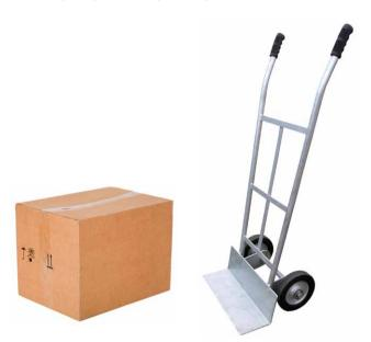
Simple machines have very few parts; compound machines are made up of two or more simple machines. A moving dolly is one example of a compound machine. It has combined two simple machines. The handles are levers that help lift the load, and the wheel and axle help move the load forward easily. The same principle applies to a wheelbarrow.
