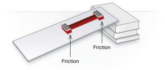
3. A ramp will be needed to test the first two principle models, B1 the sliding model and B2 the rolling model. Build a simple ramp by using books for height and a plank of wood or piece of stiff cardboard for the ramp.
