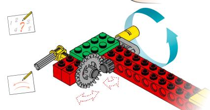
Crown gear Spur gear
