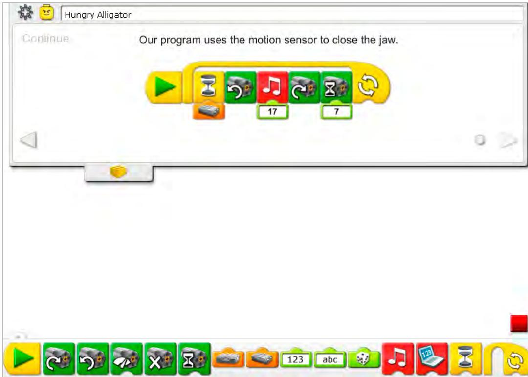
The Hungry Alligator program is modified to change the Start On Key Press to a Start Block and to add the motion sensor input. After you click the Start Block, the program waits for the motion sensor to see something. Then it turns on the Motor That Way to close the jaw and plays Sound 17, the Crunch sound. Then the motor turns on this way to open the jaw. The motor runs for seven-tenths of one second and turns off. The program repeats.
