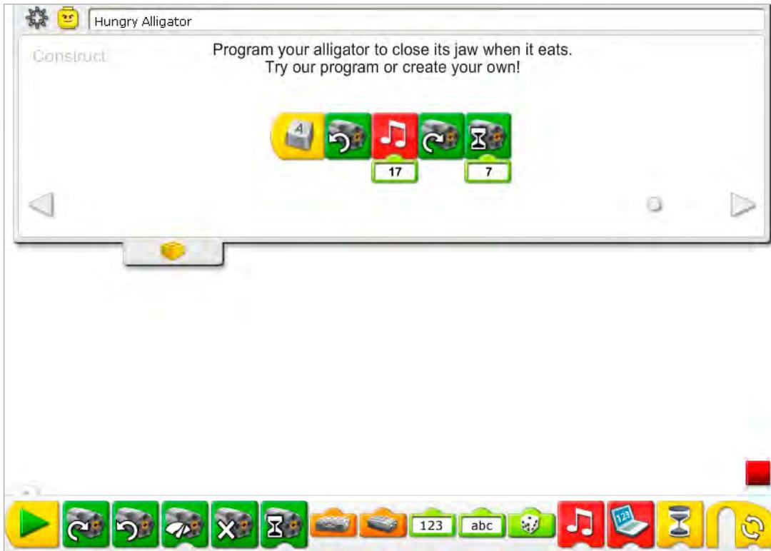
The Hungry Alligator program uses the keyboard controls to start the movement. The Start On Key Press Block waits for you to press the **A** key on the keyboard. Then it turns on the Motor That Way (counterclockwise) to close the jaw. Next, the program runs Play Sound 17, the Crunch sound. Then it turns on the Motor This Way to open the jaw. The motor runs for seven-tenths of one second and turns off.
